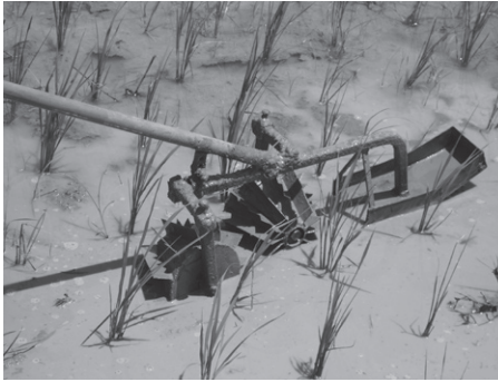
Photo 7. The churning of the soil by the weeder boosts plant growth
